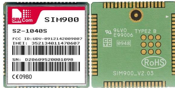
Figure 8: Top and Bottom View of the SIM900 (Arduino Channel)
