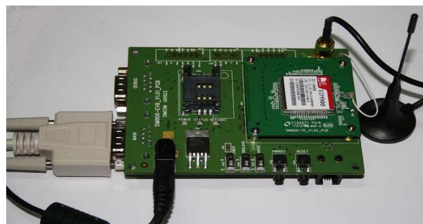
Figure 7: SIM900 Evaluation Board (Arduino Hardware)
